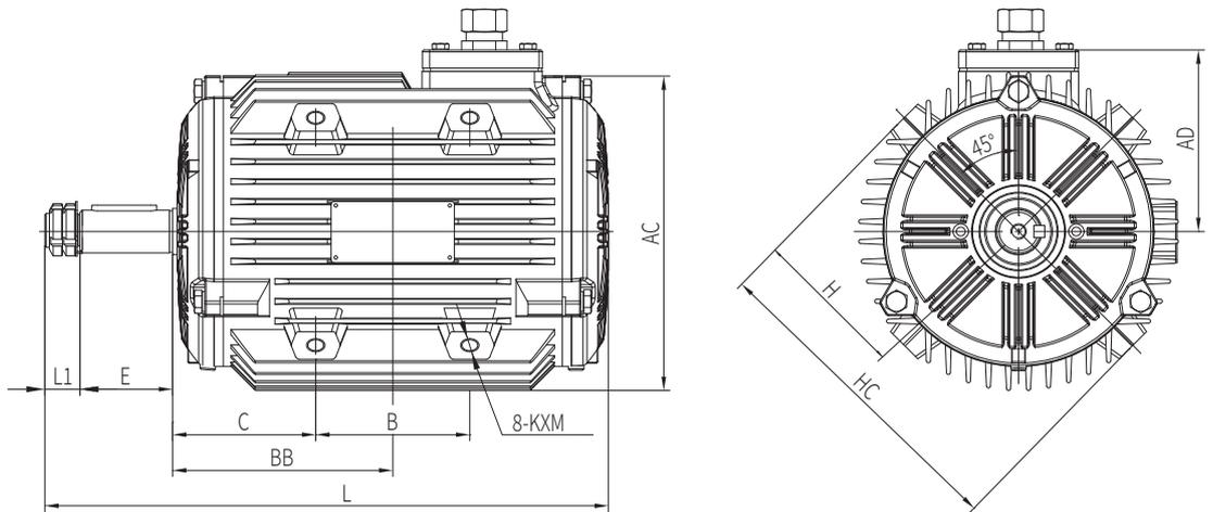
WXF3&WXF2 Foot (PAD) mounted - frame sizes 71 to 280
